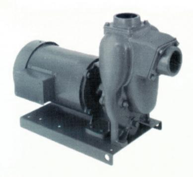
FLOMAX 5 self-priming centrifugal pumps are capable of creating vacuum sufficient to lift liquids from heights up to 25' above the source. Once primed the pumps built-in flapper valve will maintain a full column of liquid in the suction line.
